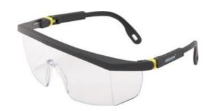
Safety glasses with black nylon frame and black temples with yellow stripe. This glasses perfectly fit to every user thanks to adjustable lenght and tilt of temples. Large clear polycarbonate lens which are made from one piece are anti-fogging, anti-scratching, resistant to low-energy shocks (up to 45 m/s) at extreme temperatures ( $-5 ^{\circ}\text{C} - +55 ^{\circ}\text{C}$ ) and provide maximum protection.
