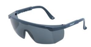
Safety glasses with dark blue nylon frame and temples. This glasses perfectly fit to every user thanks to adjustable lenght of temples. Large smoke polycarbonate lens which are made from one piece protect against UV radiation, fulfill the function of a sunglass filter, still preserve satisfactory colout perception and are resistant to low-energy shocks (up to 45 m/s) at extreme temperatures (-5°C - +55°C). They provide maximum protection and extremely wide field of vision.
