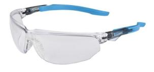
Lightweight protective glasses with unique solution of temples. Temples are made from nylon ang have a hinged system. Adjustable temple length and angle - length can be adjusted to three positions. The nose bridge is soft and ventilated. Glasses are comfortable and versatile. Clear visor is anti-fogging, anti-scratching and resistant to low-energy shocks (up to 45 m / s) even at extreme temperatures (-5  $\degree$  C - + 55  $\degree$  C).
