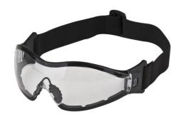
Goggles of innovative solution. Visor is panoramatic with excellent wide field. The rubber band is adjustable and 25 mm wide. The nose bridge is soft and provides excellent comfort. Goggles are very light and flexible. Clear visor is anti-fogging and anti-scratching, protects against UV radiation and it is resistant to low-energy shocks (up to 45 m/s) at extreme temperatures ( $-5 ^{\circ}\text{C} - +55 ^{\circ}\text{C}$ ).
