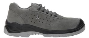
PU2D sole is antiwriting, resistant to oils and fuels and contact heat up to 110°C. It is antistatic and absorbes shocks up to 20 J in the heel area. Design of the sole provides high adhesion to the surface and the profile significantly reduce the risk of slip. Wide comfort sole reduce the feeling of tiredness, without steel toecap.
