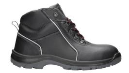
PU2D sole is antiwriting, resistant to oils and fuels and contact heat up to 110°C. It is antistatic and absorbes shocks up to 20 J in the heel area. Design of the sole provides high adhesion to the surface and the profile significantly reduce the risk of slip. Wide comfort sole reduce the feeling of tiredness.
