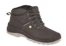
PU2D sole is antiwriting, resistant to oils and fuels and contact heat up to 110°C. It is antistatic and absorbes shocks up to 20 J in the heel area. Design of the sole provides high adhesion to the surface and the profile significantly reduce the risk of slip. Wide comfort sole reduce the feeling of tiredness.
