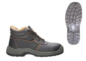
PU2D sole is antiwriting, resistant to oils and fuels and contact heat up to 110°C. It is antistatic and absorbes shocks up to 20 J in the heel area. Design of the sole provides high adhesion to the surface.
