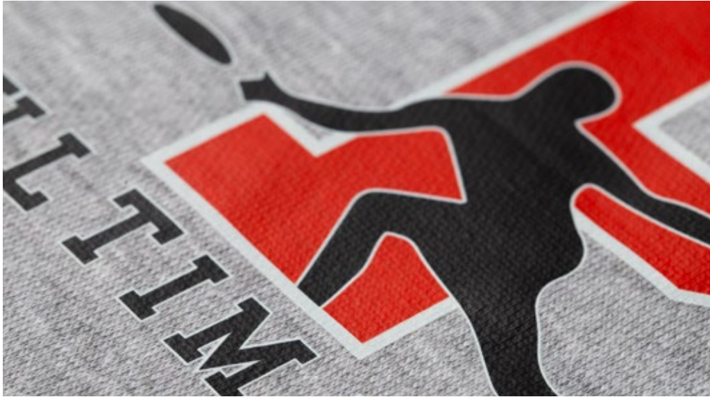
Transfer DTF (Direct To Film - Přimo na fólii). DTF prenos (Direct To Film - Priamo na fóliu).
